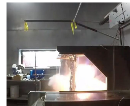
An Amerex kitchen system extinguishing a fryer fire
